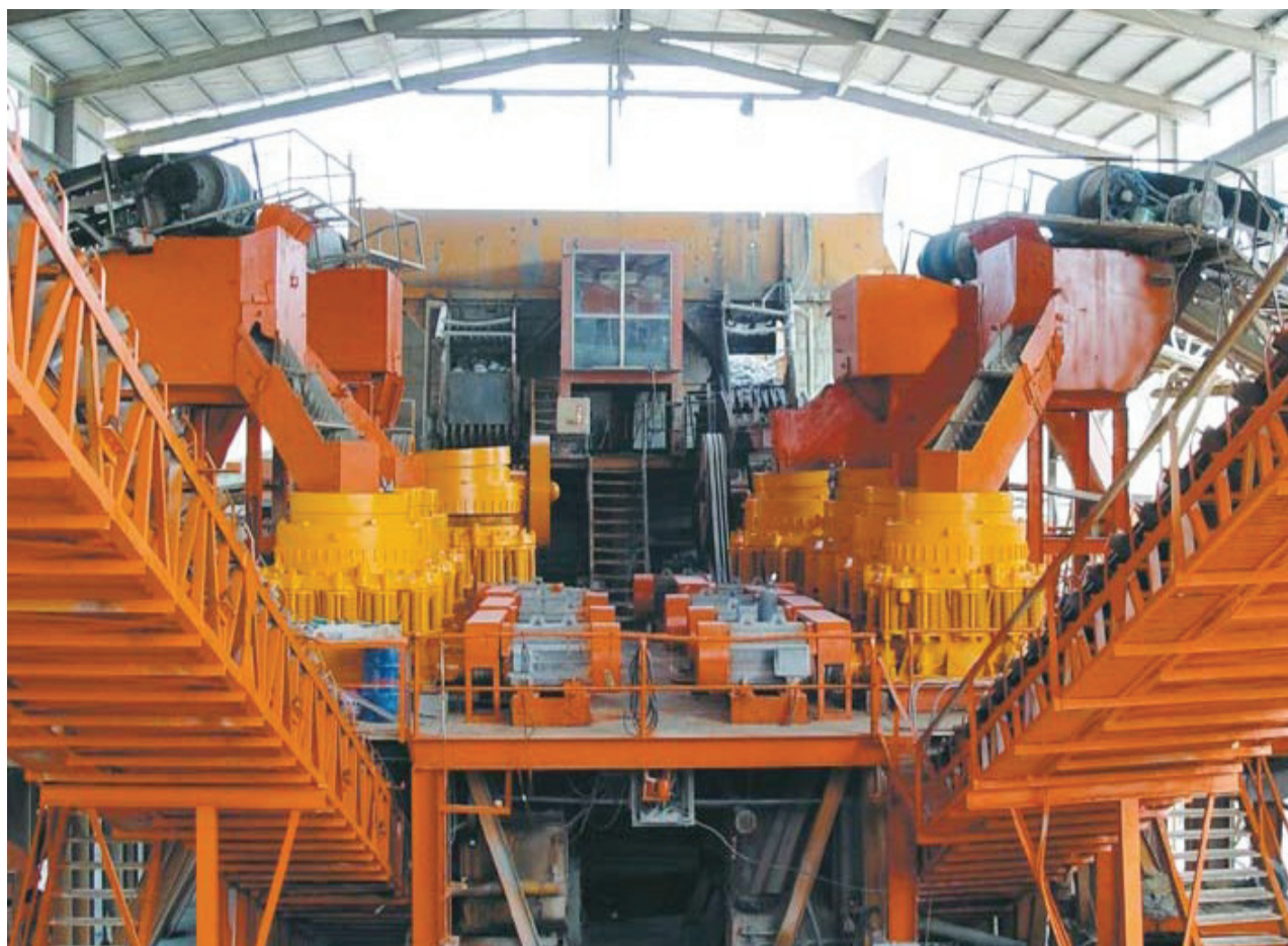
Two Production Lines each at 400TPH Throughput with Minyu Crushers in Central Taiwan.
