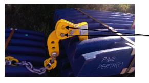
These holes allow the jaw liner to hang at different angles to facilitate liner installation.
