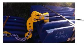
These holes allow the jaw liner to hang at different angles to facilitate liner installation. Typically, the front hole will allow the jaw liner to hang vertically.
