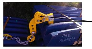
These holes allow the jaw liner to hang at different angles to facilitate liner installation. Typically, the front hole will allow the jaw liner to hang vertically.
