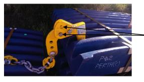
These holes allow the jaw liner to hang at different angles to facilitate liner installation.
